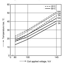
1.-(2) Coil temperature rise (200mW type) Sample: ALE74B12, 6 pcs. Point measured: coil inside
